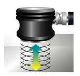
The use of different probes offers the capability to perform thickness measurements in inaccessible surfaces, on very thin plates, on high temperature environments, above paint (thru-coat or echo to echo functions) as well as on surfaces with intense local corrosion without any surface smoothing required (use of pencil type probes).
