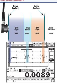
The 25 MULTI PLUS calculates and simultaneously displays thickness measurements of up to four individual layers. It also displays total thickness of selected layers.
