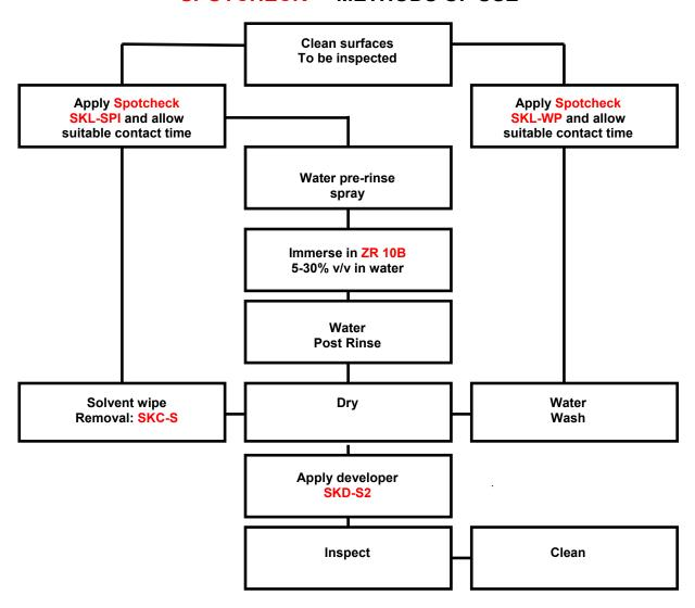
Colour contrast red dye penetrant is used throughout industry for the detection of surface defects Penetrants give clear vivid red indications of surface flaws, easily seen by the naked eye.
