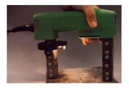
The light source and leg assembly, which is activated by the magnetic field, it switches on automatically during testing. Ideal for darker corners. Pt No 002L115
