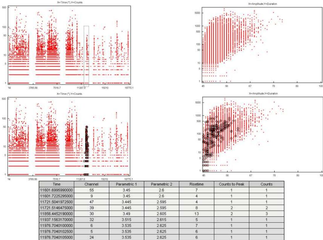
An Example of the mouse select action on a point plot. The upper graphs are typical graphs in AEwinPost. The user has selected some data dragging the mouse over the data (dashed rectangle). The selection is shown on the lower graphs. Part of the selection is visible on the Hit Table (greyed hits). A selection is visible in this manner in all data graphs, waveform graphs and tables. The data selected can be removed (deleted) by just pressing the Del button.
