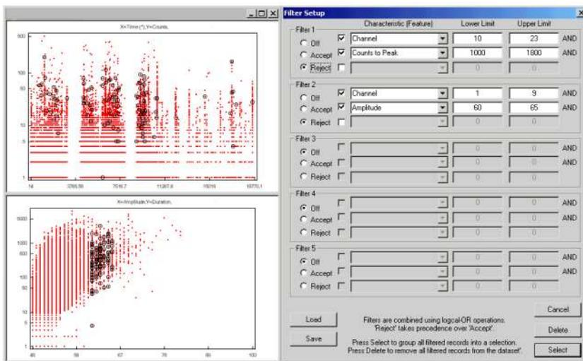
*Typical filtering action using the Data Filters dialog. A complex filter has been set-up and applied to the data. The results can be seen as a selection on the two graphs so that the user can review the effect of the filter before deleting any data.*
